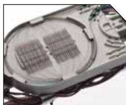
Loose Bufer Tube Storage
